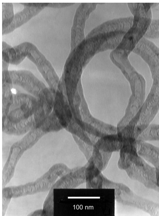
Fig. 22. TEM image of the multiwalled CNTs, obtained with 15 sccm CO 2 carrier gas.
