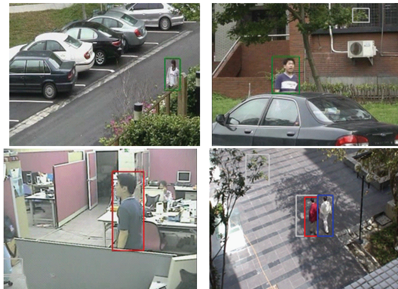
FIGURE 18: The processed results for some occlusion cases.
