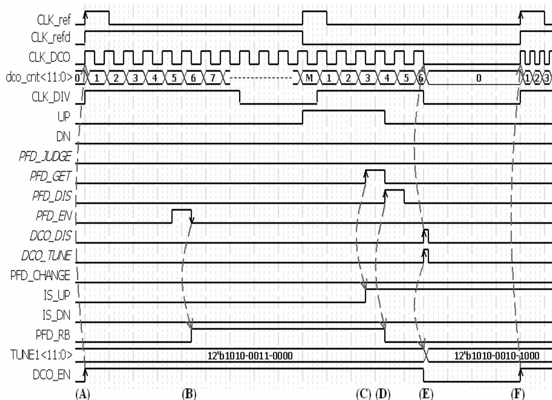
Fig. 3.14. The timing diagram of SAR frequency search state
