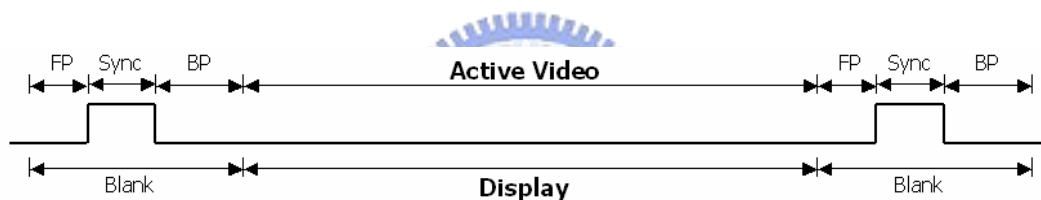
Fig. 2.3. Video synchronous signal timing definition
