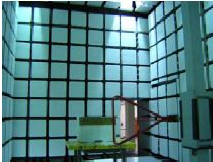
圖3.16 2D anechoic chamber
