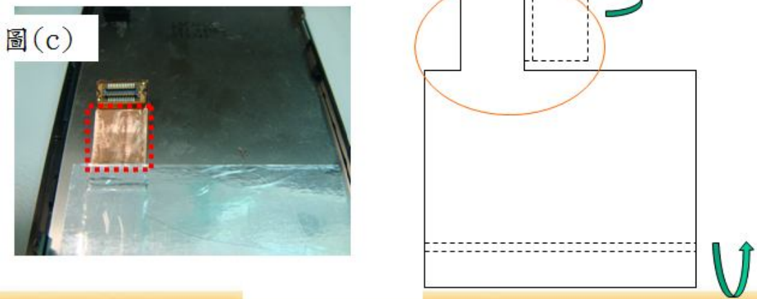
圖3.21 銅箔解決2G/3G wireless sensitivity方案
