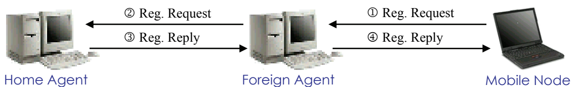
Figure 3 Registration in Mobile IP
