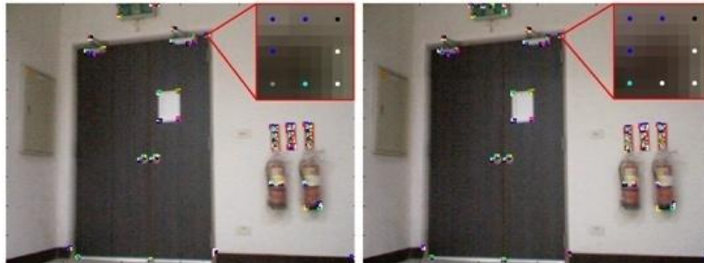
Figure 5.7 A pair of stereo images of an indoor scene overlaid with color codes of corner feature points.
