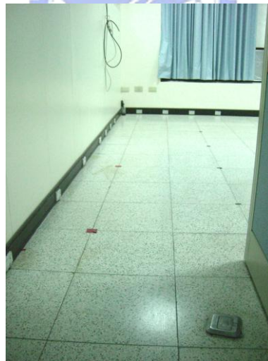
Figure 4.3 The scene which provides real data that used in our experiments. The reference points attached on the wall are co-planar. The size of each tile is 40\text{cm} \times 40\text{cm} .
