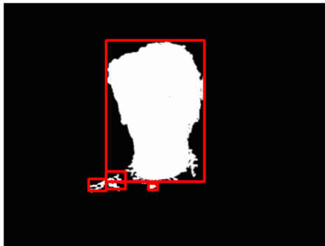
(c) The result of removing regions of small sizes and improper shapes in (b).
