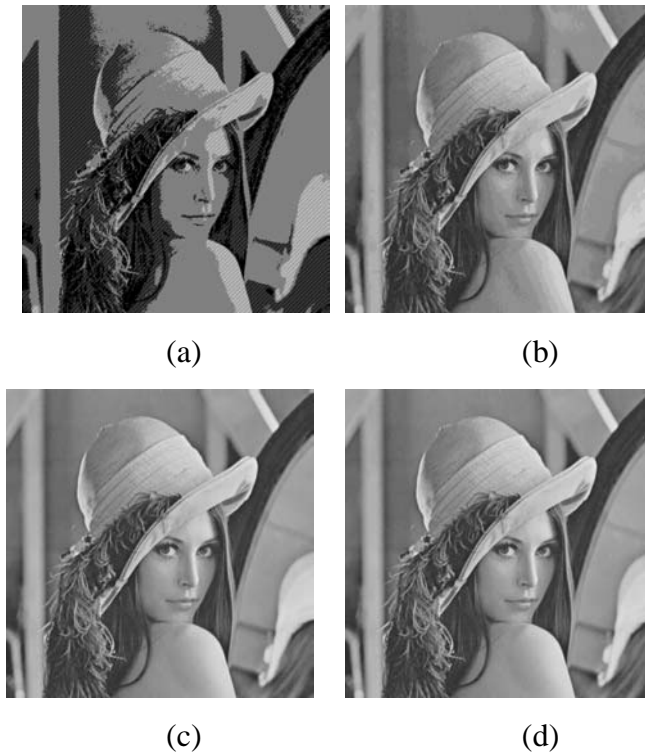
Figure 2.5. The recovered images revealed from various numbers of stego images. (a) from any 2 stego images (PSNR=14.57); (b) from any 3 stego images (PSNR=29.28); (c) from any 4 stego images (PSNR = 48.46); (d) from any 5 stego images (lossless).
