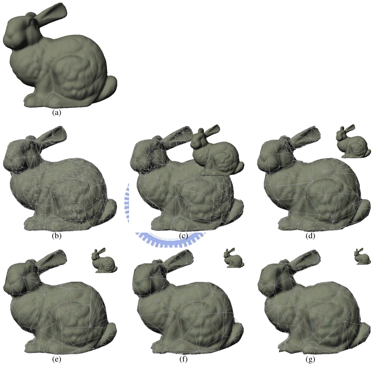
Figure 5.6: (a) is the original mesh (65,491 polygons) of a bunny viewed at one cell away (cell size 50), (b-g) are MVMeshes of the bunny at 1 (1,605 polygons), 2 (945), 3 (554), 4 (392), 5 (330), 6 (306) cells away. The upper-right indicates actual projected images.
