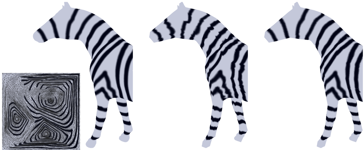
Figure 3.16: Textured images of horse model. Left: original model of 8160 polygons with parameterized texture map, center: simplified model of 800 polygons without texture adaptation, right: simplified model of 800 polygons with texture adaptation.
