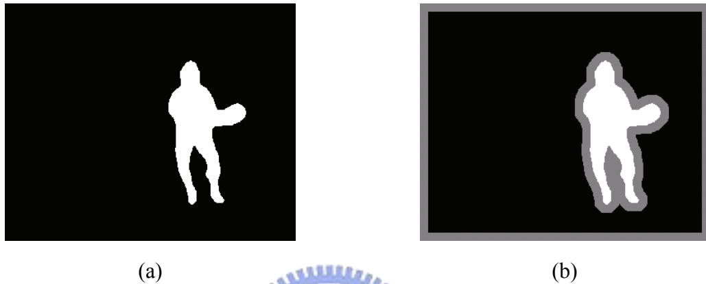
Fig. 1.4 Reliability mask used in the reliability-based blending. (a) Segmentation mask. (b) Reliability mask derived from (a).
