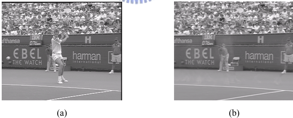
Fig. 2.1 Object blurring effect of averaging blending. (a) Original frame. (b) Reconstructed background of (a).
