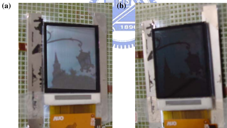
Fig. 6-25. Demonstrated photographs of a directional backlight with an LCD panel at the positions of (a) left and (b) right eye.
