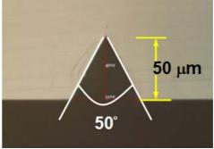
The photos of fabricated micro-grooves in anisotropic foils with pitch of 200  $\mu$ m and vertex angle of 50°.
