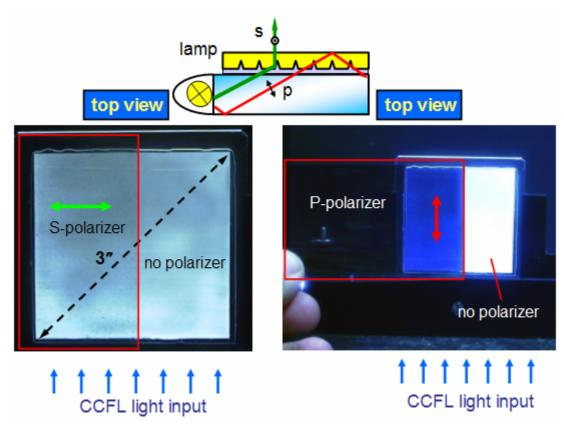
The luminance profiles of S-polarized and P-polarized light by rotating the polarizing direction of polarizer.
