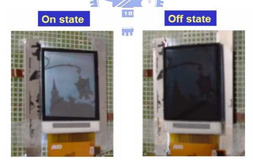
The demonstrated on-state and off-state photos of the directional backlight with LC panel while only left-handed light source switching on.
