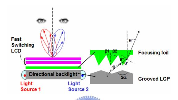
The configuration of time-multiplexed 3D displays composed of a directional backlight with a fast switching LCD.
