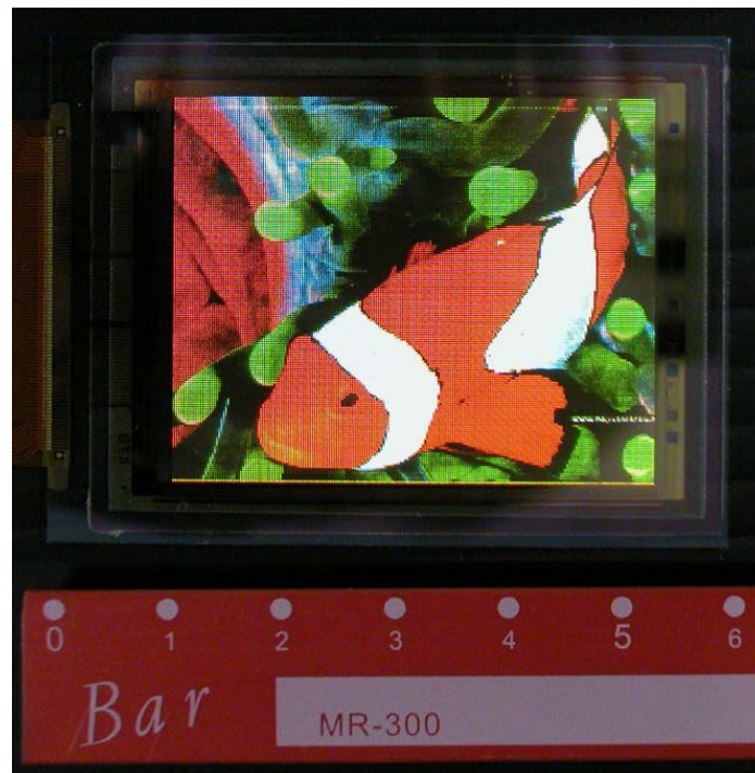
Fig. 5-23. A color photograph taken directly from the current-driven AM-OLED display panel.
