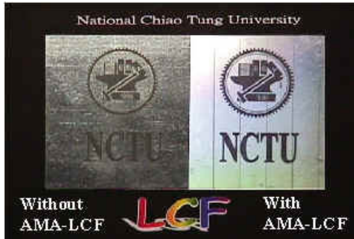
Fig. 4-2. Example photograph of unidirectional AMA-LCF used for brightness enhancement.
