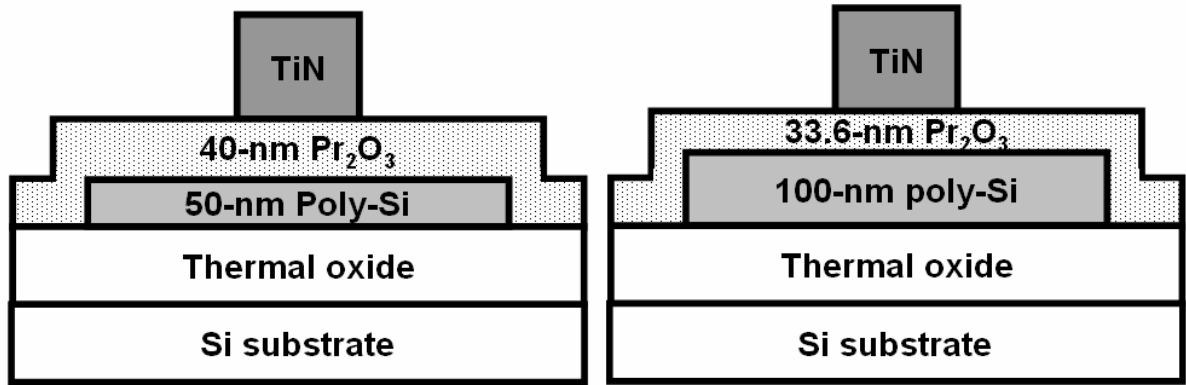
(d-1) 40-nm \text{Pr}_2\text{O}_3 deposition, densification, and TiN gate formation.
