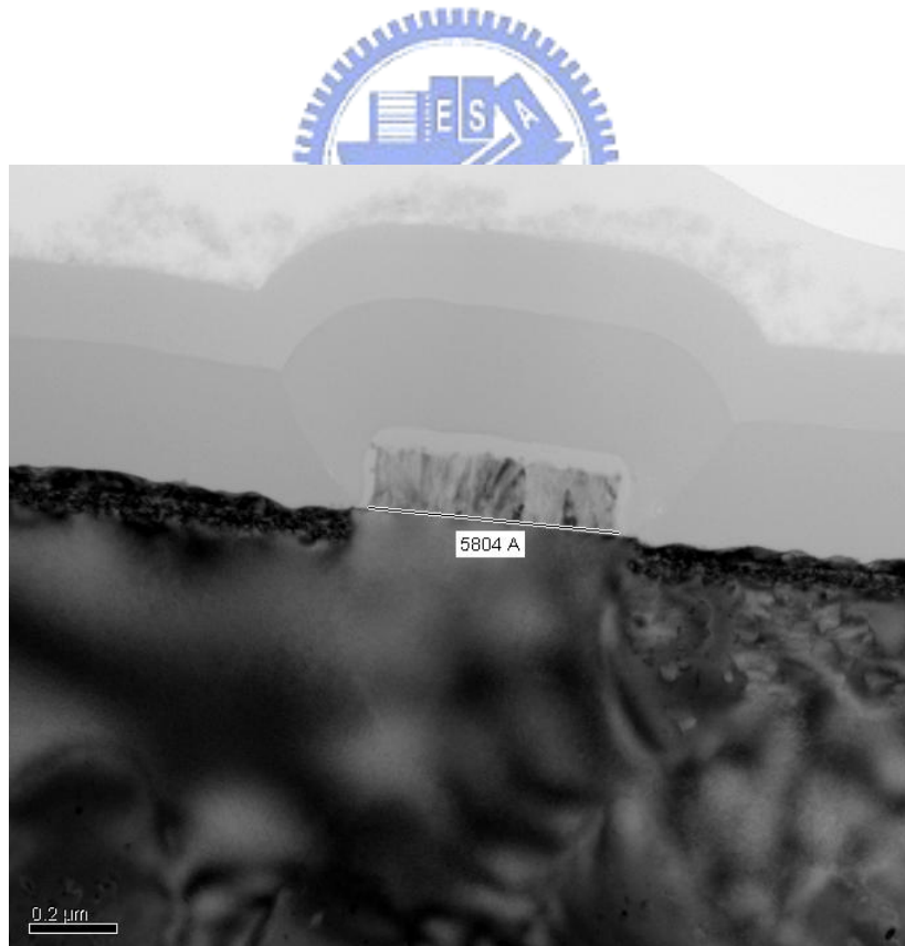
Fig. 2.1 Schematic cross section of the local strained channel PMOSFET
