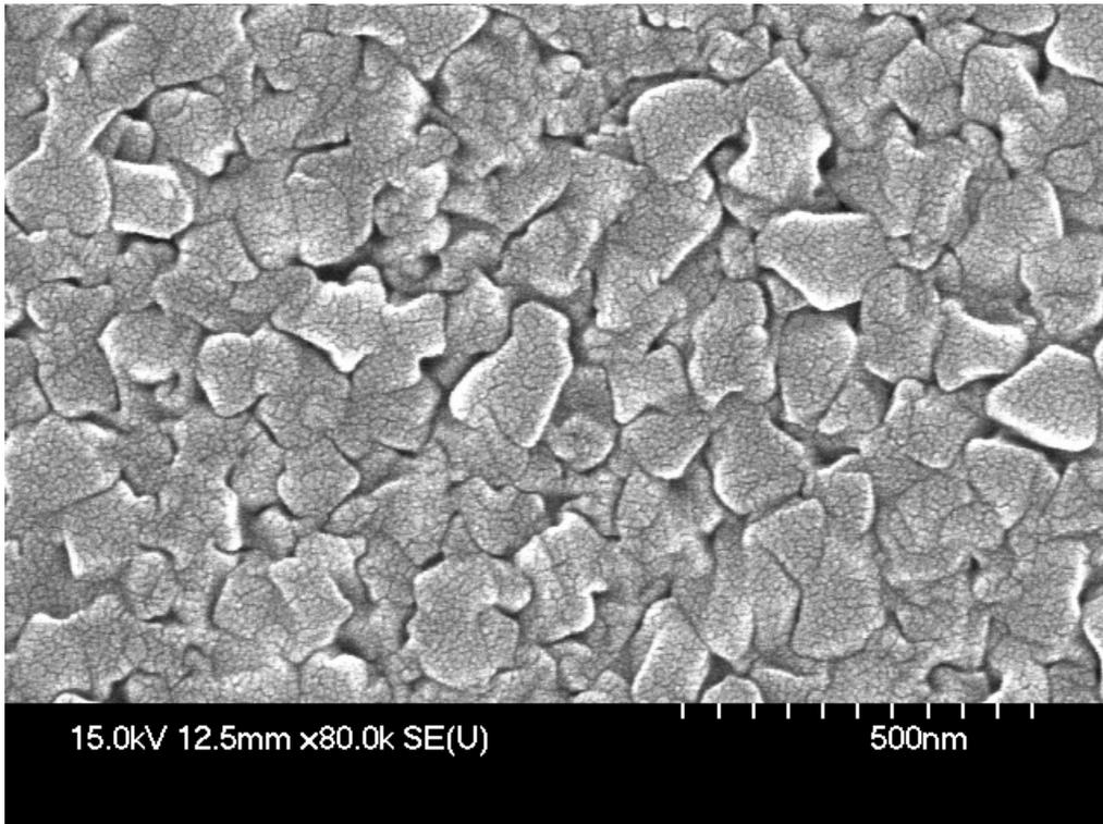
Fig. 4-11-3 SEM image of the 1wt% grown AZO film at  $T_s = 250^\circ\text{C}$ .
