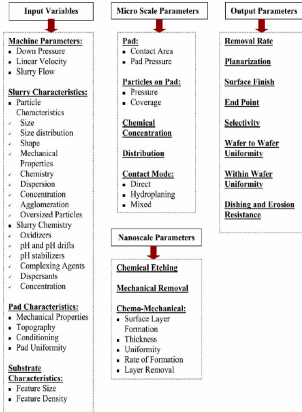
Figure.1-4 Interacting factors in a CMP process.
