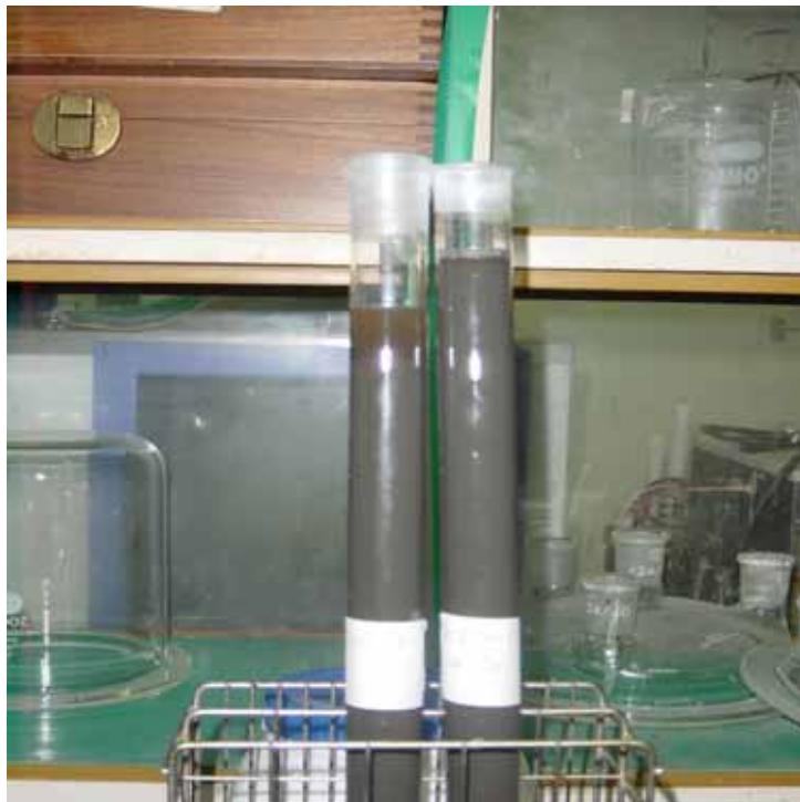
Figure 53 導電粉體抗沈降測試
