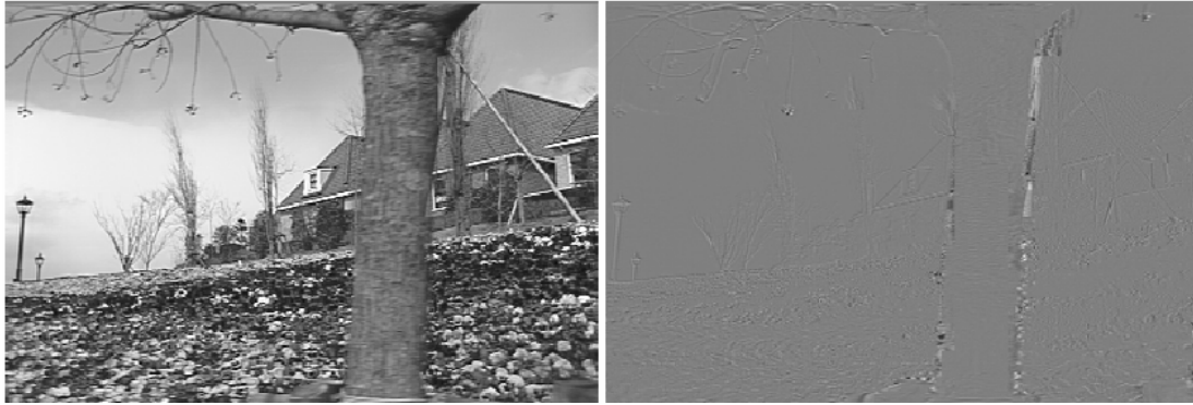
Figure 2-4 Temporal filtering with motion compensation (left: low pass, right: high pass).
