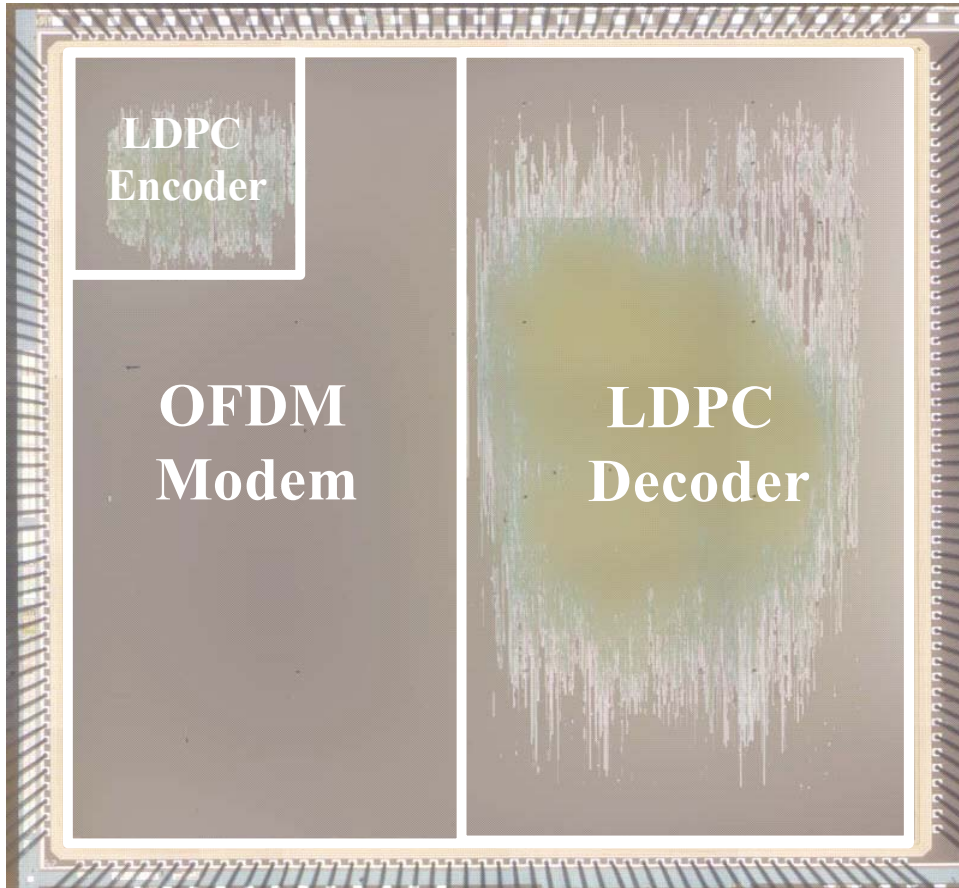
Fig. 4.13 Die micrograph of the LDPC-COFDM UWB transceiver chip
