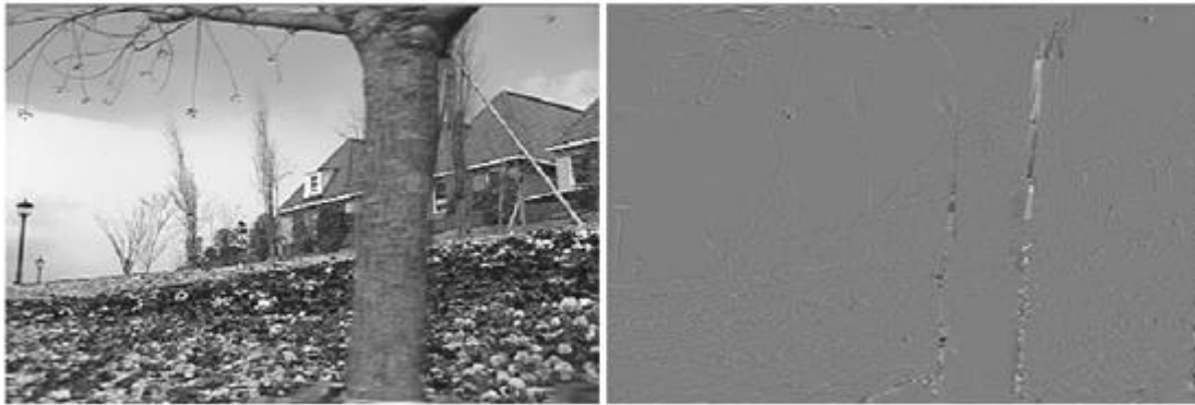
Figure 2.7: Temporal filtering with motion compensation. Left: low-pass frame. Right: high-pass frame
