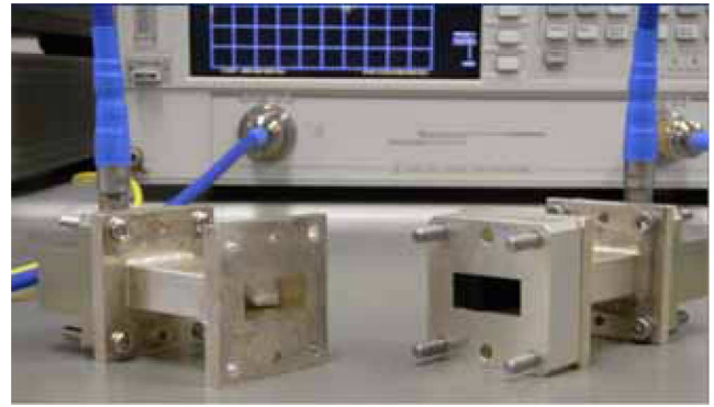
Fig. 14. X-band waveguide (WR-90) measurement system.
