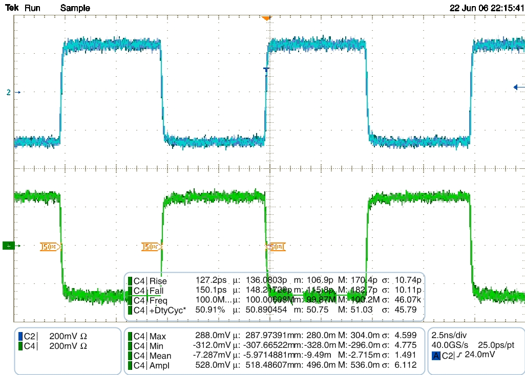
Fig. 5.49 Measurement of differential output from DIVIDER
