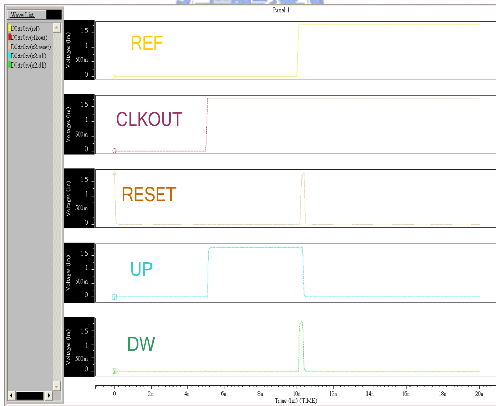
Fig. 5.10 Timing diagram of PFD
