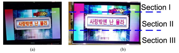
Fig. 26. (a) The power consumption of LCD panel with color filter and CCFL backlight is larger than 5 W. (b) The power consumption of the color filterless LCD panel with the proposed RGB backlight driver is about 2-3 W.
