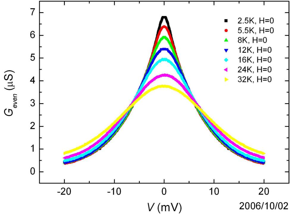
Figure 4.15:  $G_{even,data}(V, T)$  as a function of  $V$  at several temperatures.
