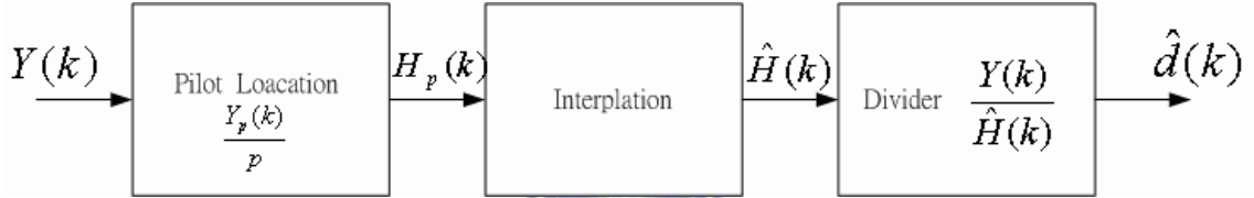
Figure 4.2: Channel estimation steps.
