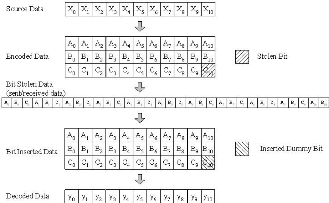
figure 2.2.5 11/32 coding rate bit-stealing and bit-insertion procedure (source : 802.15.3a proposal)
