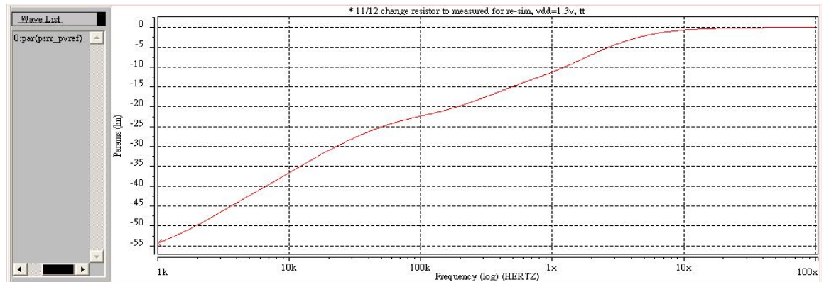
Fig. 5-22 Simulated PSRR of Type C under typical condition axis X : frequency (Hz) ; axis Y : PSRR of p-Vref (dB)
