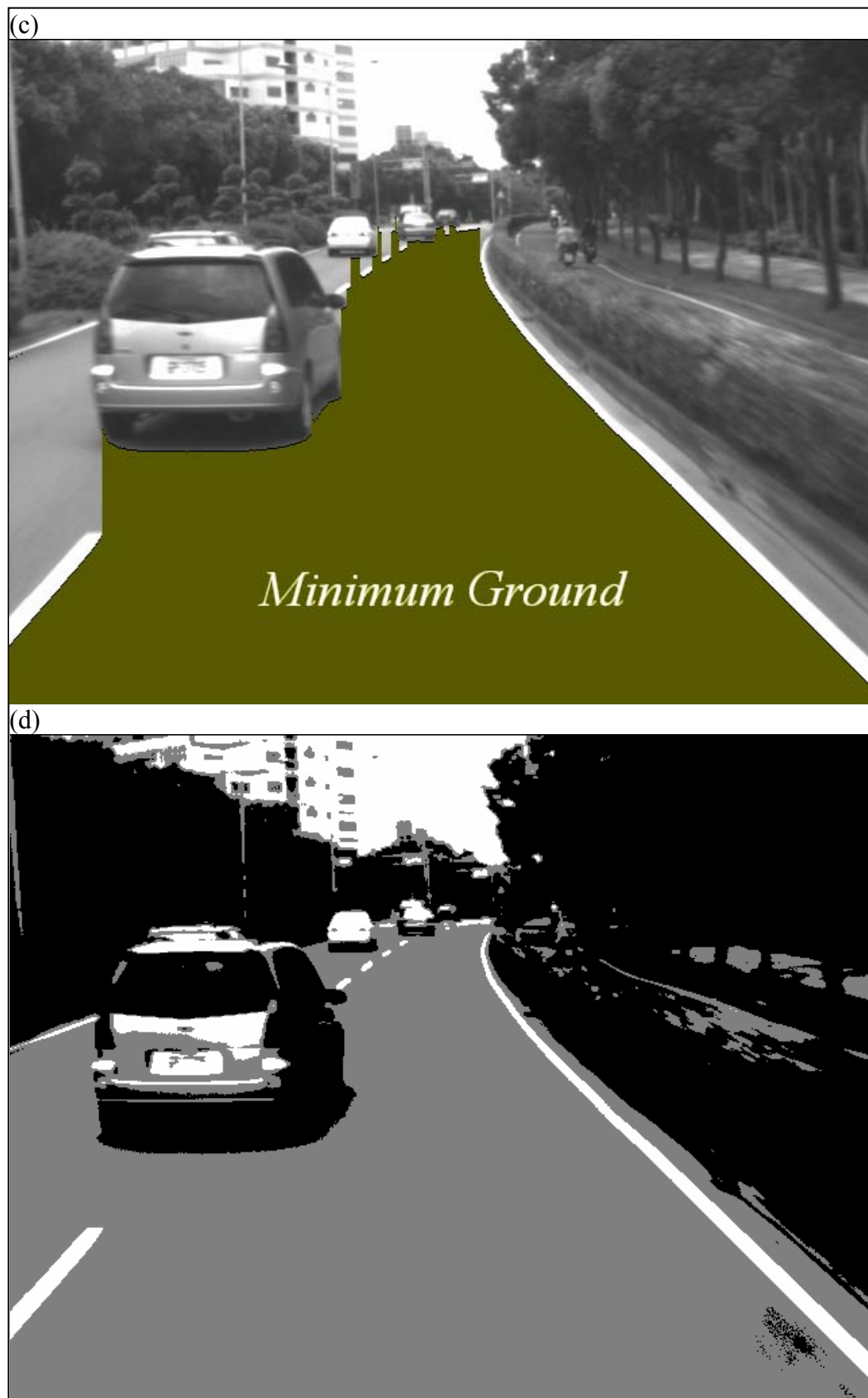
Fig. 3.12 An example of the preprocessing. (c) The road image with the Minimum Ground . (d) After the second image segmentation without the Minimum Ground .
