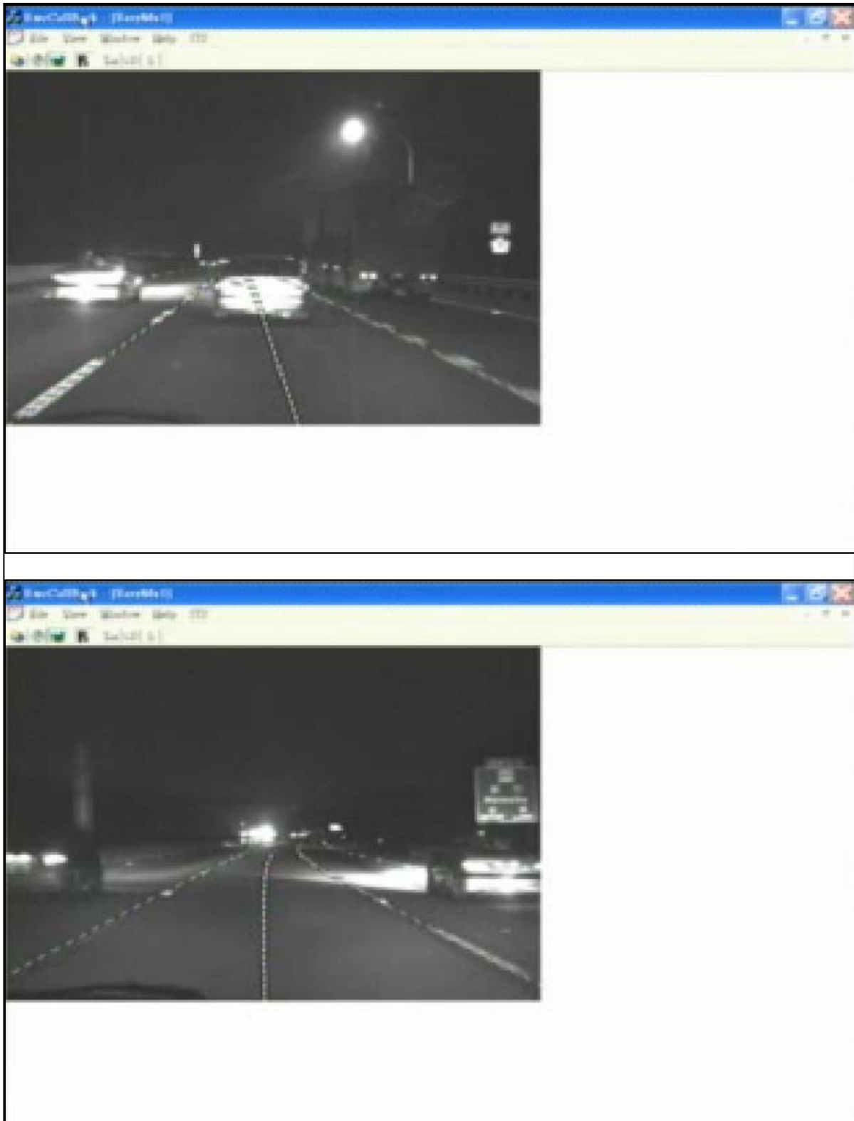
Fig. 5.12 Results of the real-time lane detection on the freeway by night.
