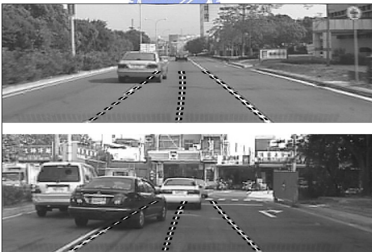
Fig. 5.7 Results of lane detection on the roads interfered with the text.
