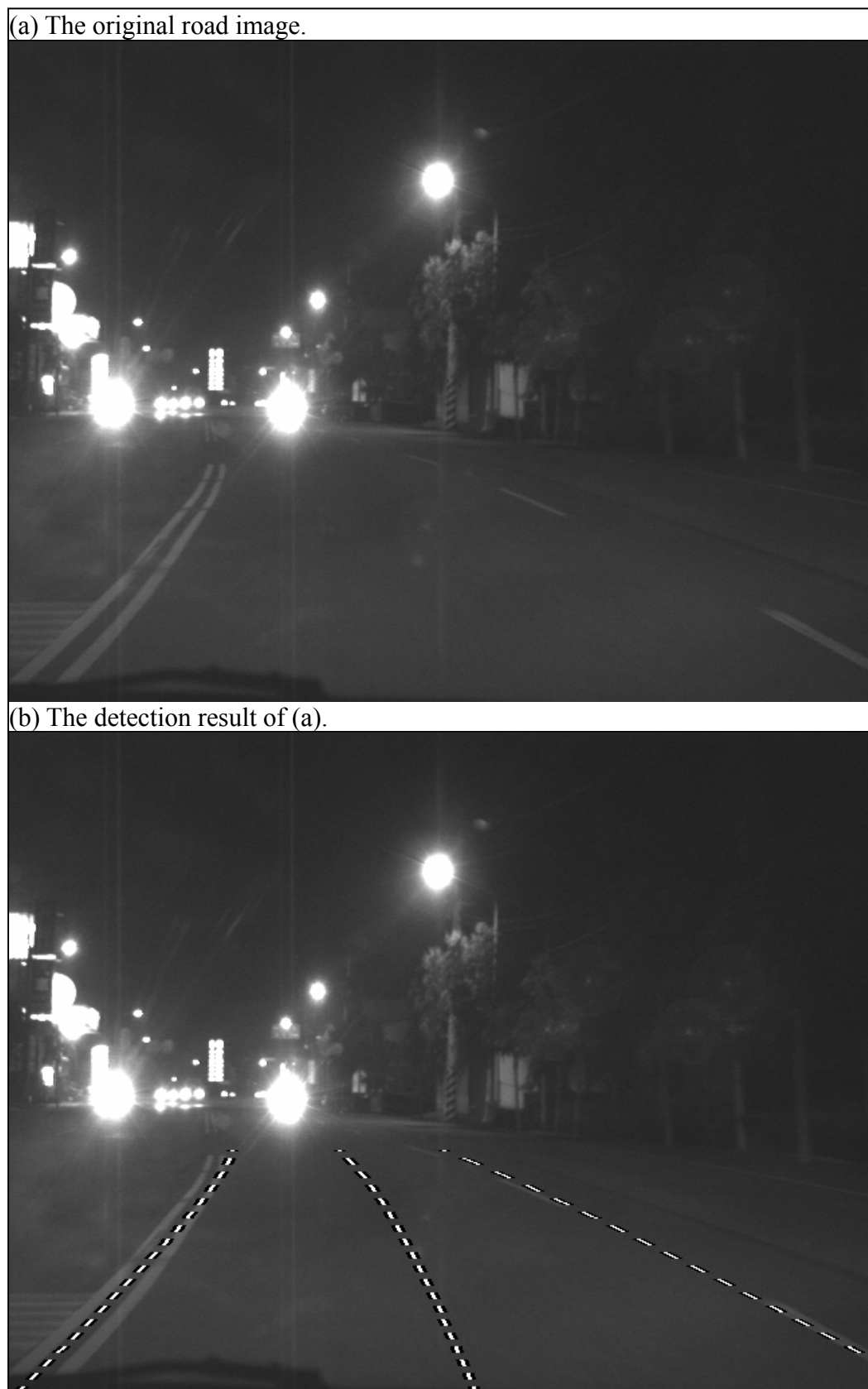
Fig. 5.9 Result of lane detection on the night road. (a) the original night road image. (b) the detection result of (a).
