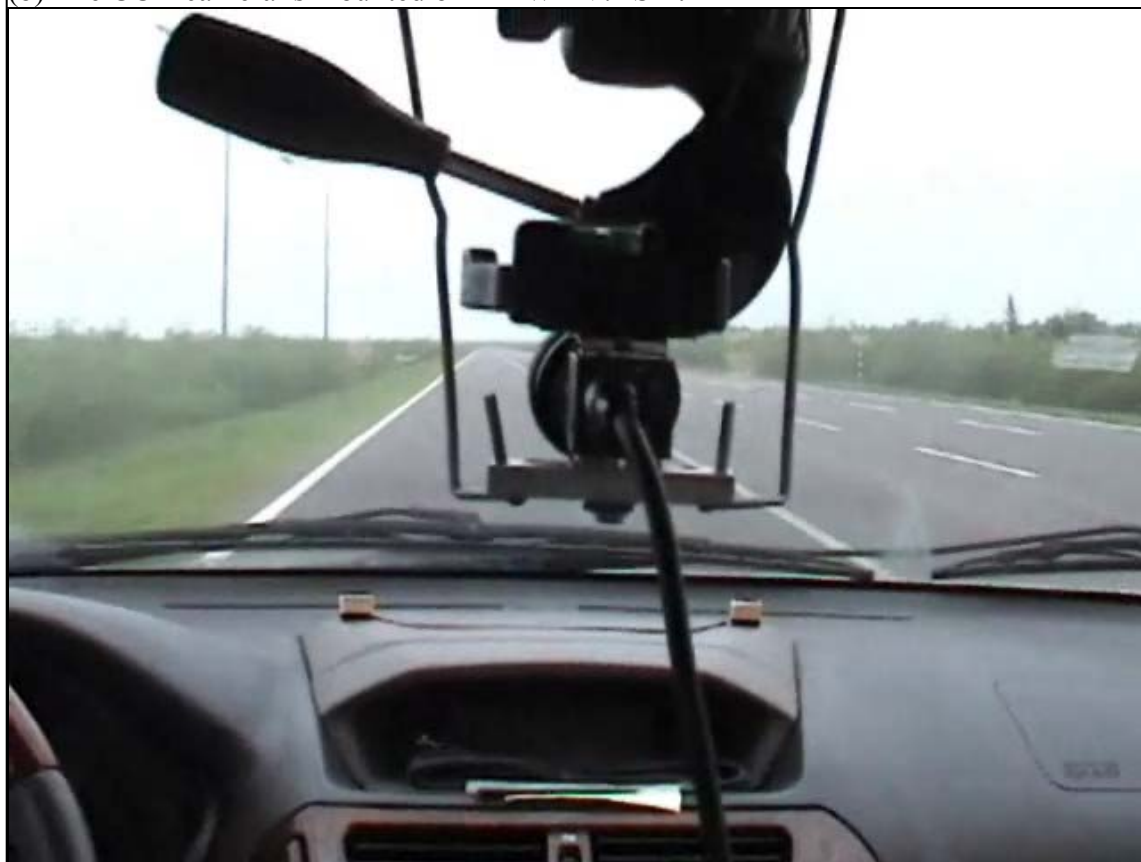
Fig. 5.13 TAIWAN i TS-1. (a) TAIWAN i TS-1 is running on the freeway under 110 km/hr. (b) The CCD camera is mounted on TAIWAN i TS-1.
