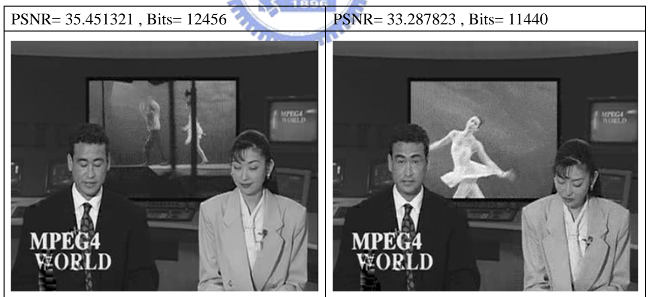
Figure 4-11 Subject view of reconstructed frame for News sequences at the 21 st frame and 146 th frame
