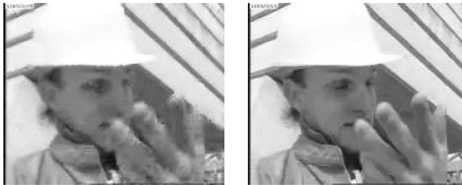
Fig 2.2: Subjective view comparison of MPEG-4 ASP (left) and H.264/MPEG-4 AVC baseline (right) at bit-rate 112Kbps. (Excerpted from [22])
