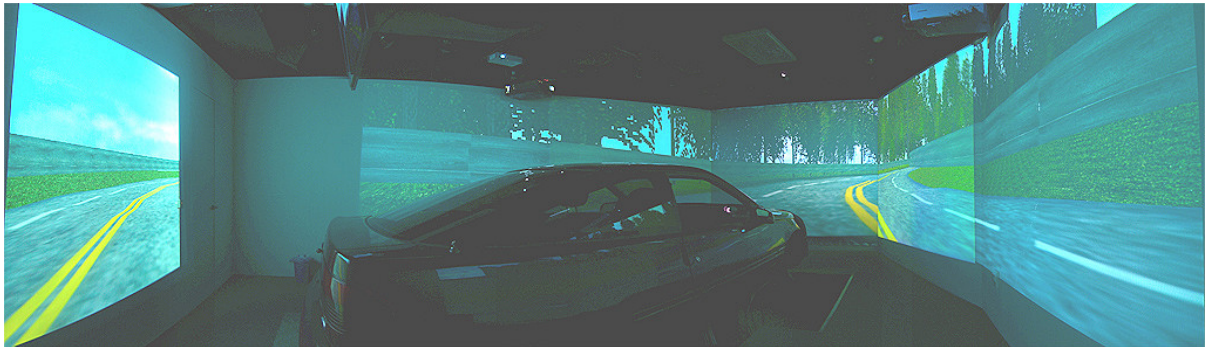
Fig. 2-3: The VR-based four-lane highway scenes are projected into 360° surround screen with seven projectors. Several photos captured from different view angle at a fixed point are connected to form this wide figure.
