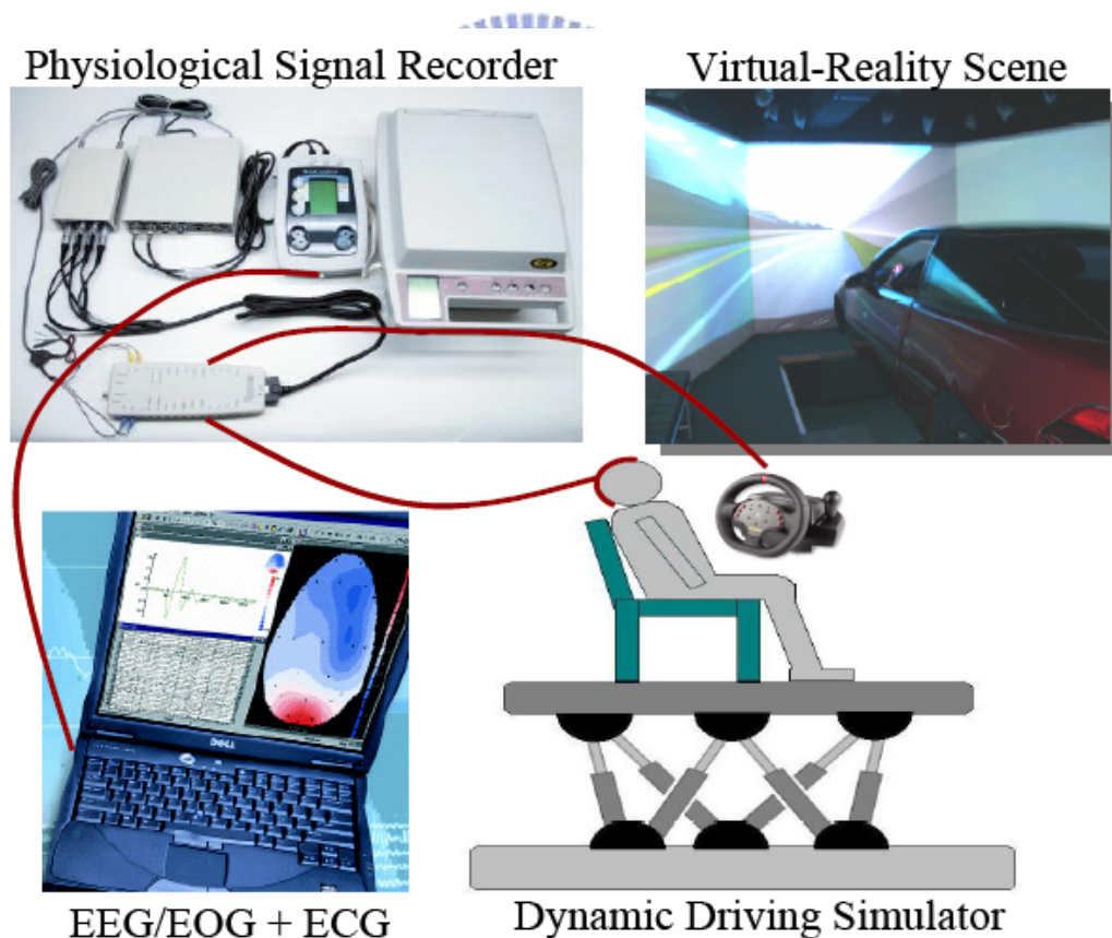
Fig. 2-1: The block diagram of the dynamic VR-based driving simulation environment with the EEG-based physiological measurement system.
