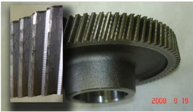
Fig. 18 Pre-shaved gear used in the experiment
