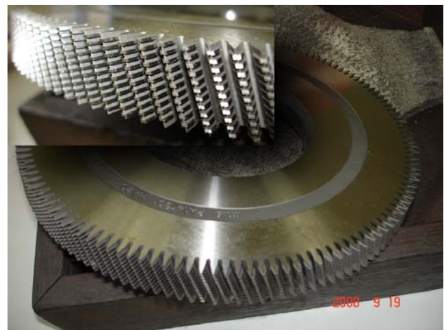
Fig. 17 Plunge shaving cutter used in the experiment
