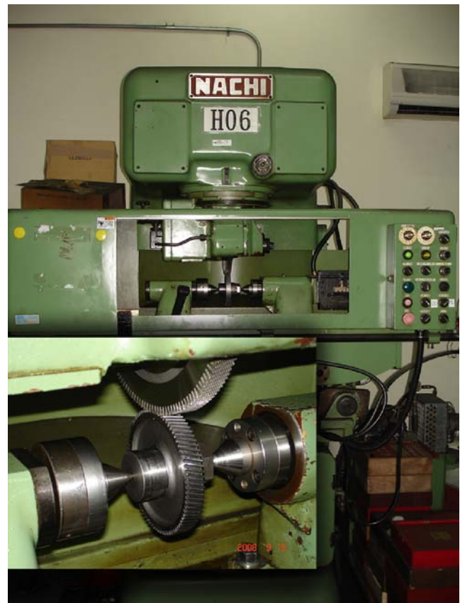
Fig. 21 NACHI shaving machine used in the experiment
