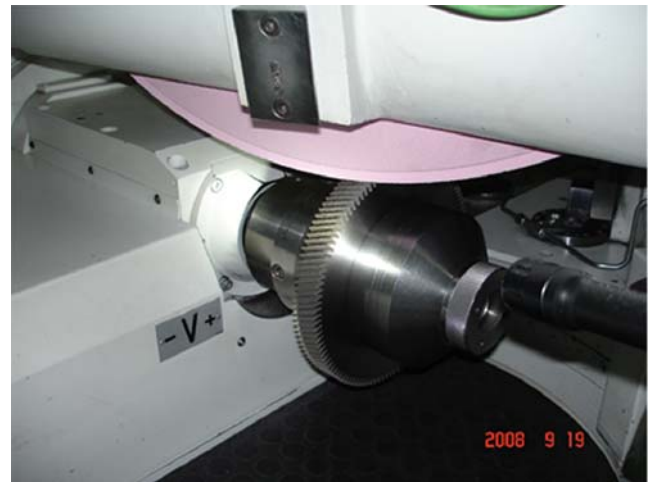
Fig. 20 Plunge shaving cutter ground by the grinding wheel of the re-sharpening machine
