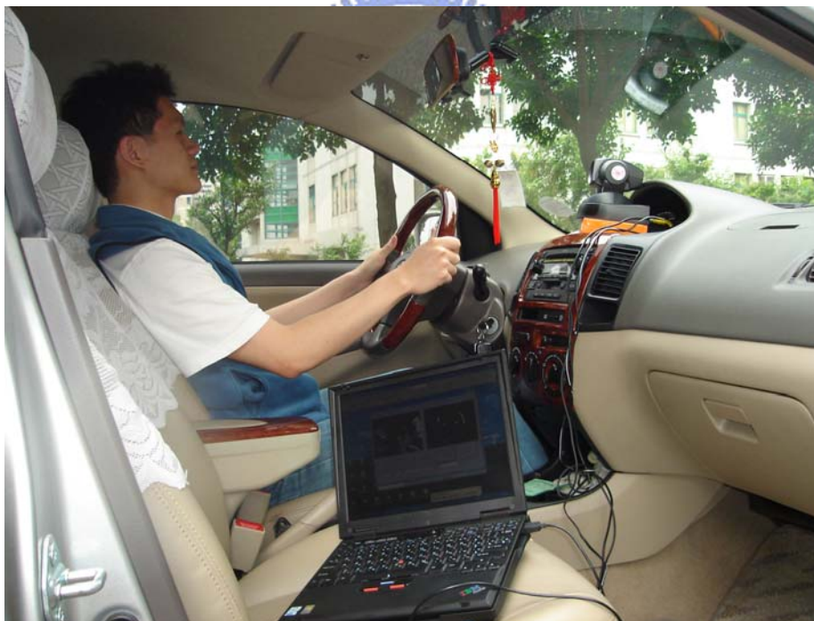
Fig. 4.13. The setups of driver drowsiness detection system: a CCD camera mounted on the dashboard and connected to a notebook.
