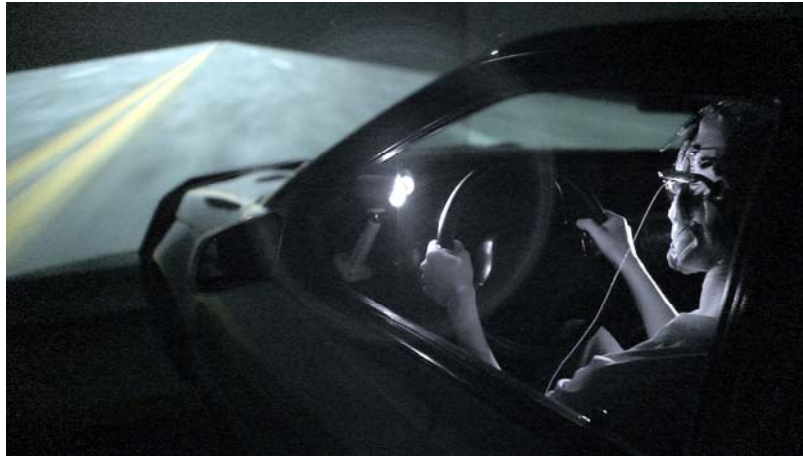
Fig. 4.5. A subject was steering the driving simulator through night-time highway scenery projected on the screen.
