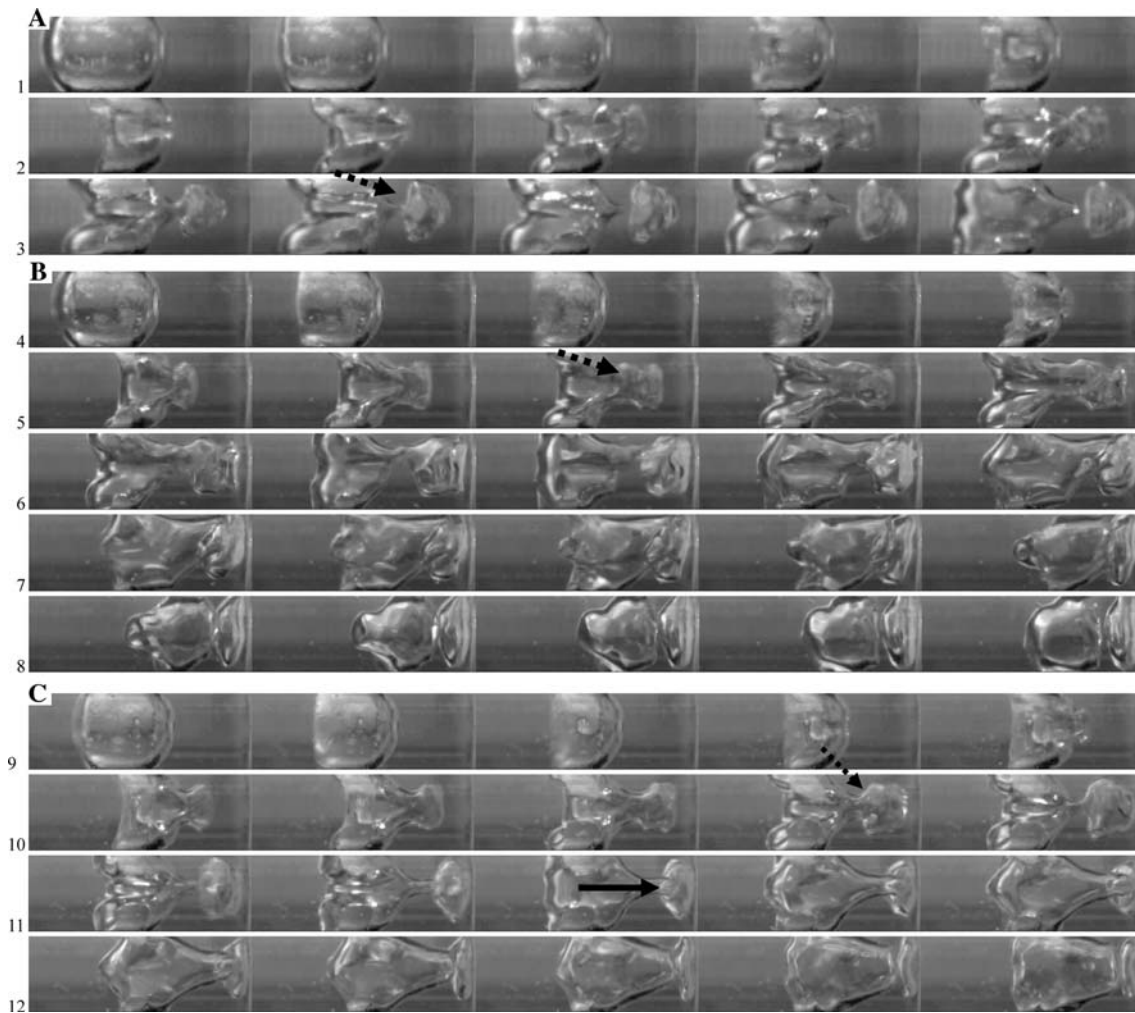
Fig. 8 Images of the process of bubble collapse at \gamma \approx 3 . The peak strength of the pressure wave for a 200 kPa, b 300 kPa, c 360 kPa. The size of each individual frame for a 10.5 \times 3.1 mm; b 9.6 \times 3.1 mm; c 9.6 \times 3.1 mm. R_{\max} for a 2.45, b 2.35, c 2.25 mm. D_j for a 1.0 mm (second image at the second row); b 0.9 mm (fifth image at the fourth row); c 0.95 mm (fifth image at the ninth row). D_{v,\max} for A : 2.5 mm (second image at the third row); b 2.0 mm (third image at the fifth row); c 2.4 mm (first image at the
