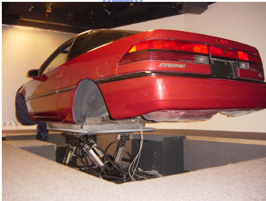
Fig. 2-10. A real car fixed on the Stewart platform.
