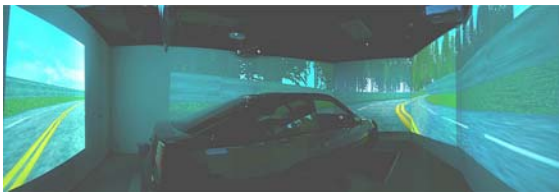
Fig. 2-2. A 360-degree 3D VR dynamic driving environment.
