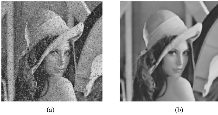
Figure 4.31. Simulation results of a 2-D RMF application. (a) The noisy “Lena” image corrupted by 9% of impulsive noise. (b) The “Lena” image processed by the 3 \times 3 RMF.
