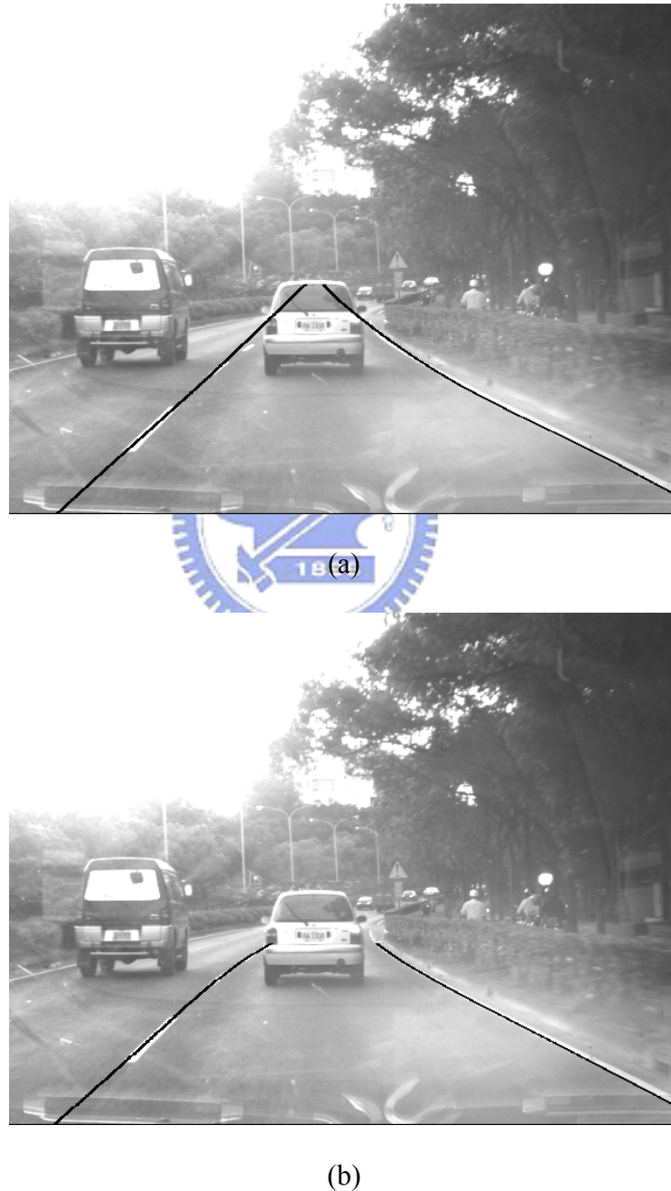
Fig. 3-24. Results of the road scene under strong sunlight. (a)Results of Jung and Kelber [46]; (b) Results of the proposed approach.
