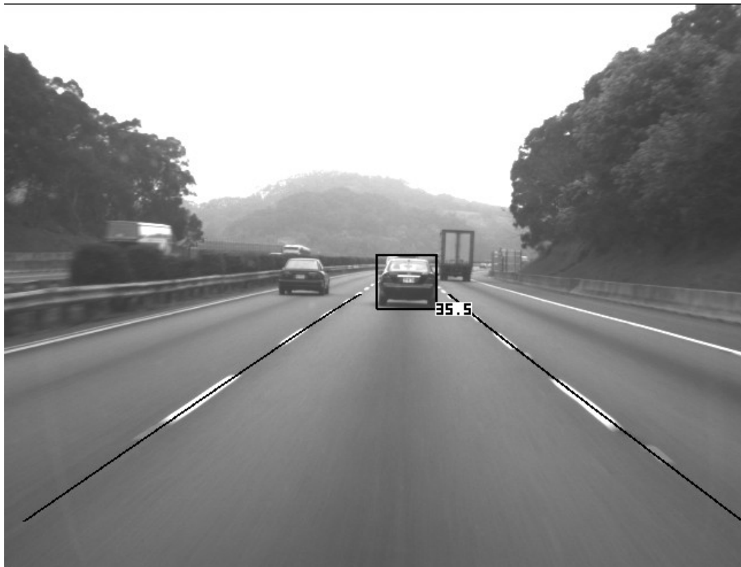
Fig. 4-9 Results of lane and vehicle detection.
