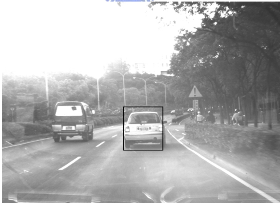
Fig. 4-7. Vehicle detection under sunny conditions.
