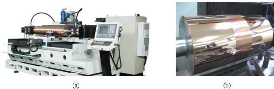
Fig. 10. Pictures of (a) our home-made drum roll lathe and (b) the roller for imprinting the BCSG.
