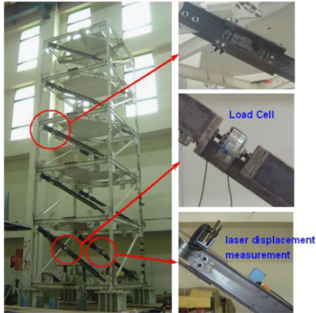
Figure 14. Experimental setup of a 5-story model frame implemented with pre-bent strips.
