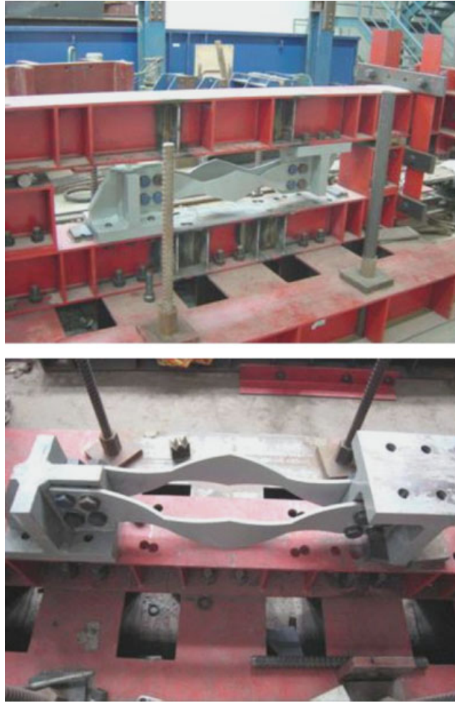
Figure 9. Experimental setup for component test of a pre-bent strip pair in a non-symmetric layout.
