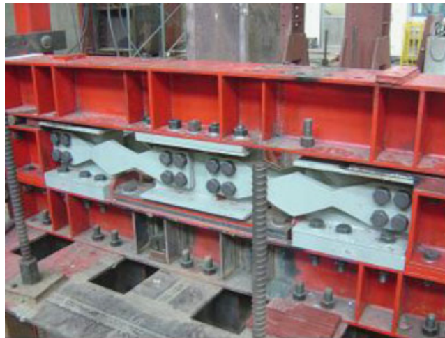
Figure 12. Experimental setup for component test of coupled pre-bent strips in a symmetric layout.
