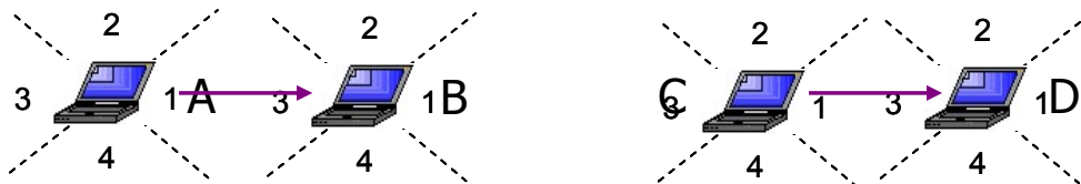
Figure 4.3: The 4-node linear topology: Node A transmits to node B and node C transmits to node D.
