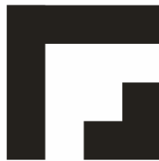
Figure 3.1: A single DSRR with the property which can increase the resonant frequency with the same lattice constant as SRR.
