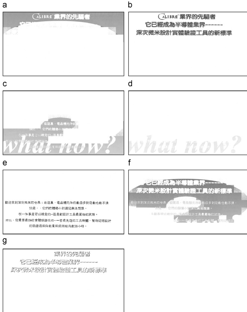
Fig. 6. An example of the test image, “Calibre”, and the object planes obtained by the multi-plane segmentation (image size = 1929x1019): (a) object plane \mathcal{P}_0 , (b) object plane \mathcal{P}_1 , (c) object plane \mathcal{P}_2 , (d) object plane \mathcal{P}_3 , (e) object plane \mathcal{P}_4 , (f) object plane \mathcal{P}_5 , and (g) object plane \mathcal{P}_6 .
