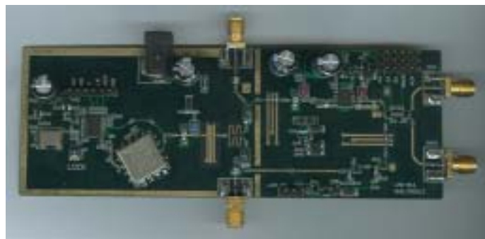
Figure 3.29 Photograph of transceiver module.
