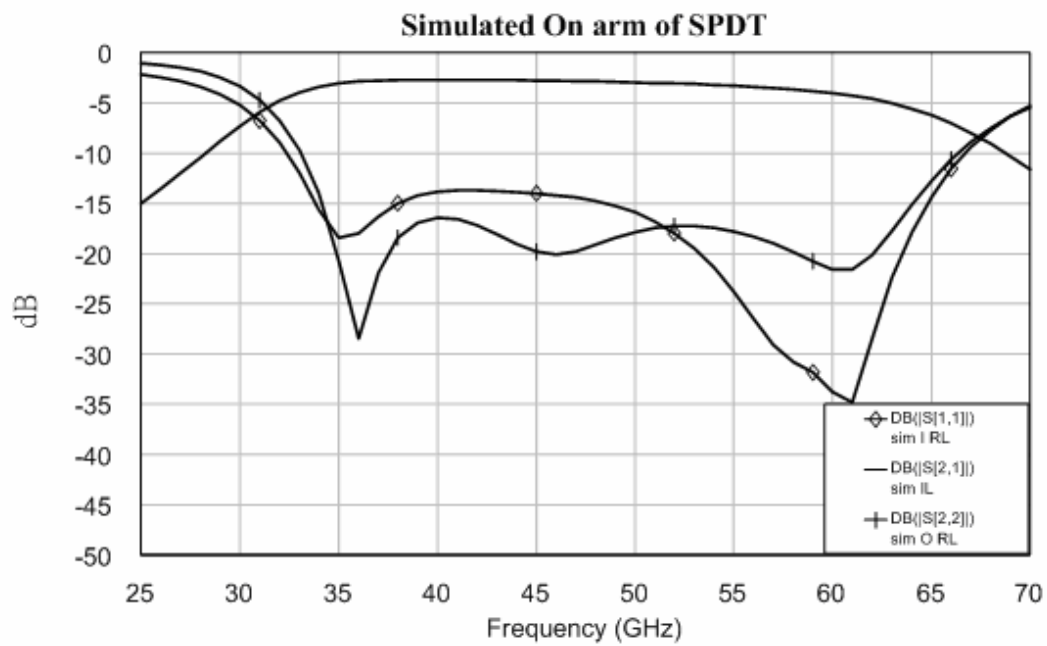
Fig. 5.6 The simulated return loss and insertion loss for the on-arm of the 33-to 60 GHz SPDT Switch
