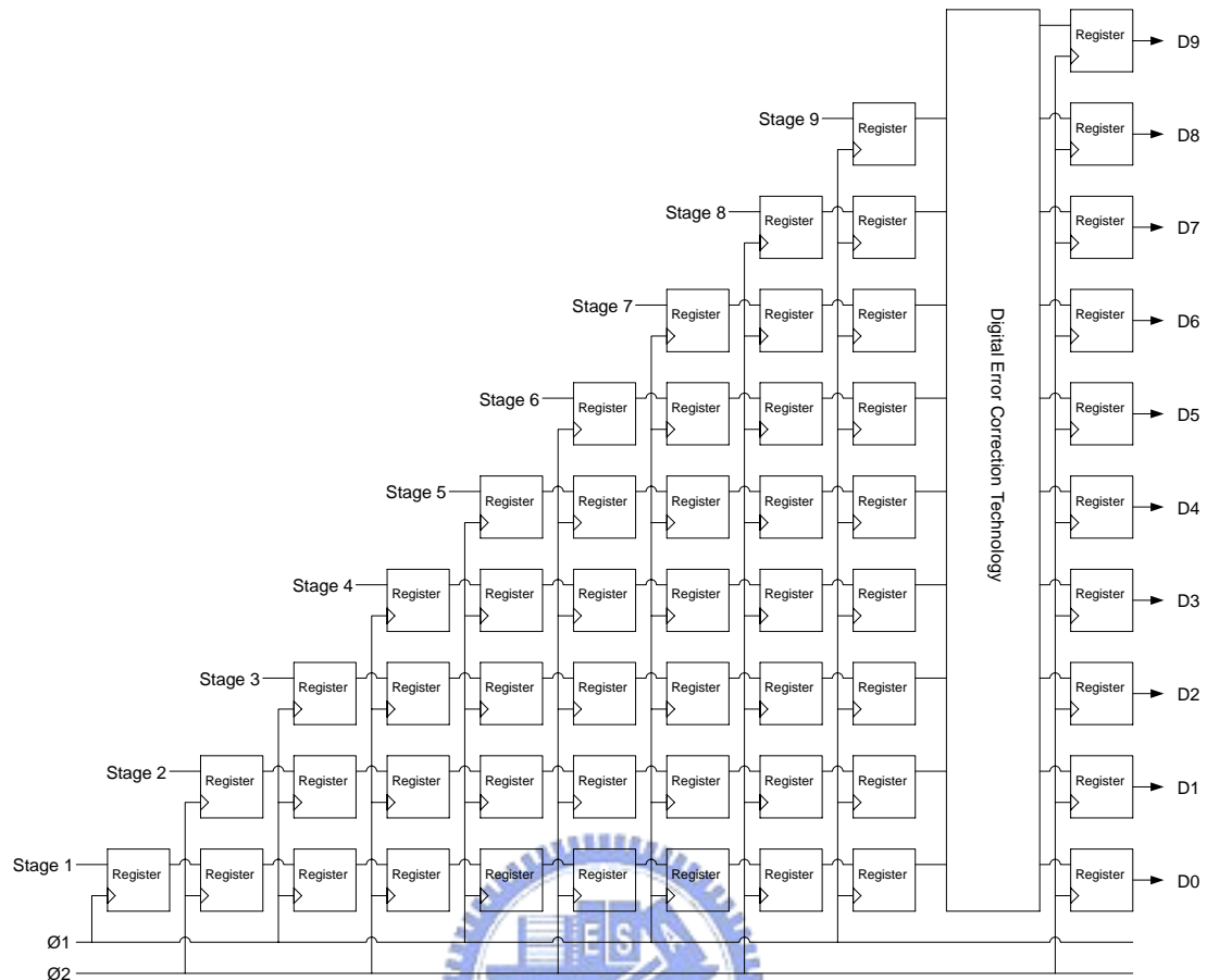
Figure 2.15 Register array of the pipelined ADC
