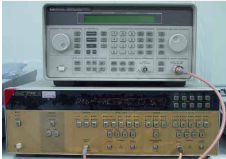
Figure 4.4 Clock generator, the top instrument is signal generator HP 8648C, and the bottom instrument is pulse generator HP 8133A
