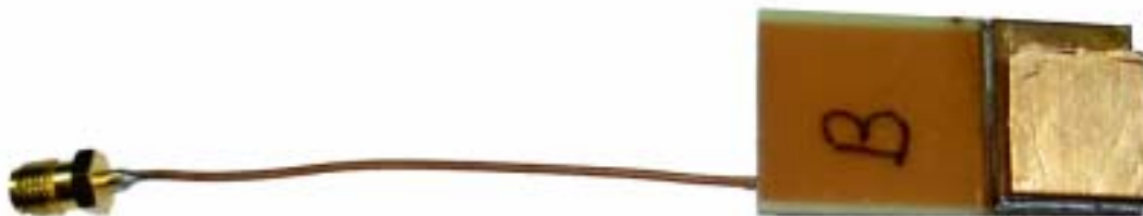
Fig 4-13 Photograph of on-package PIFA connected to BPF at the position B.
