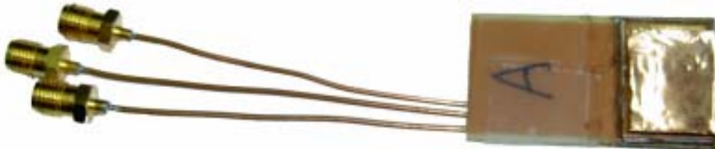
Fig 4-12a Photograph of on-package with BPF in case A.
