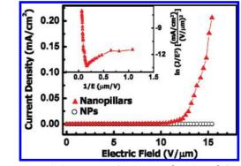
FIGURE 3. Emission current density as a function of the applied electric field on Cu nanopillars and NPs (inset: corresponding FN plots).
